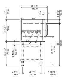
Cold Water inlet 1 (cleaning) CWII Cold Water Inlet 2 (steam CWI2
